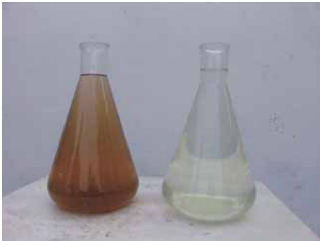
Before Treatment BOD about 200 mg/l
