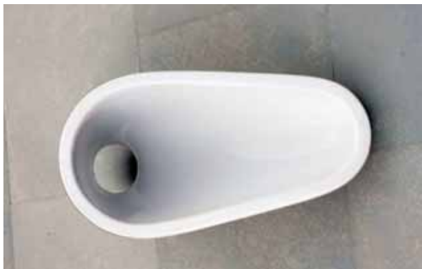
Ceramic Pan with 25° to 28° slope - it needs only 1.5 litre of water per flushing due to slope and P-trap
